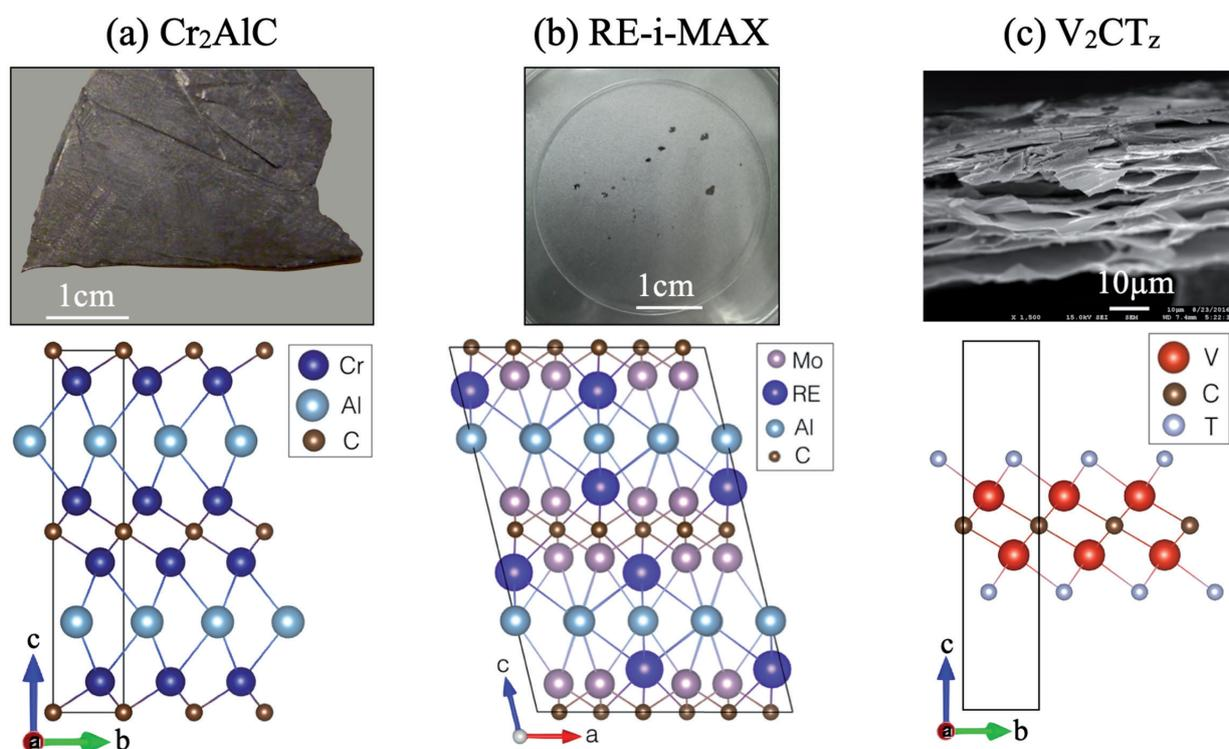
Figure 2. Materials investigated in this thesis, including 3D MAX phase single crystals: (a)  $Cr_2AlC$  and (b) RE-i-MAX, and 2D MXenes: (c)  $V_2CT_z$ .
