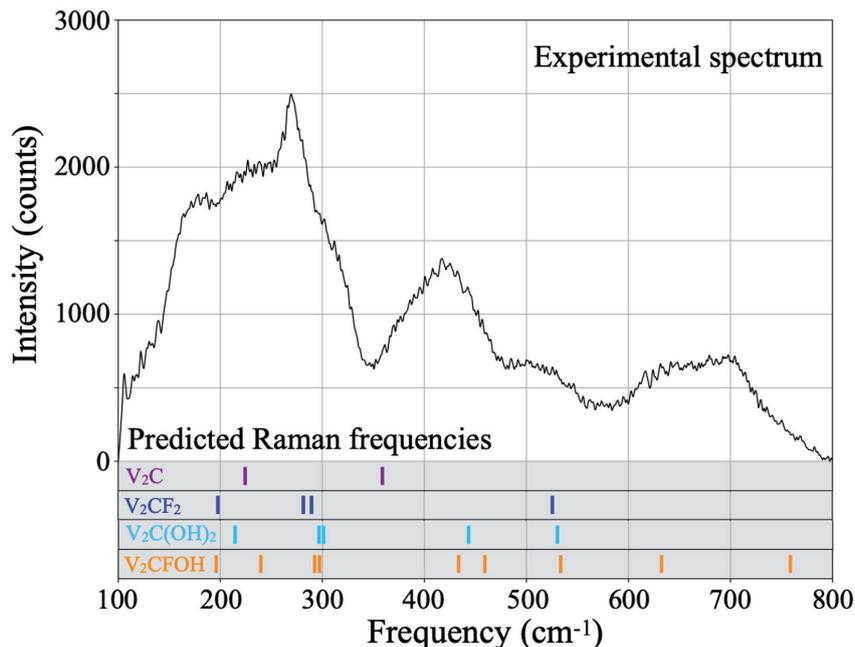
Figure 15. Raman spectrum of the exfoliated  $V_2C$ -based sample collected at RT. The calculated Raman-active frequencies of the  $V_2C$ ,  $V_2CF_2$ ,  $V_2C(OH)_2$ , and  $V_2CFOH$  mono-sheets are included under the experimental spectrum for comparison. The matching between the predicted normal-mode frequencies and the experimental spectrum confirms the presence of heterogeneous terminal groups at the  $V_2C$  surface.
