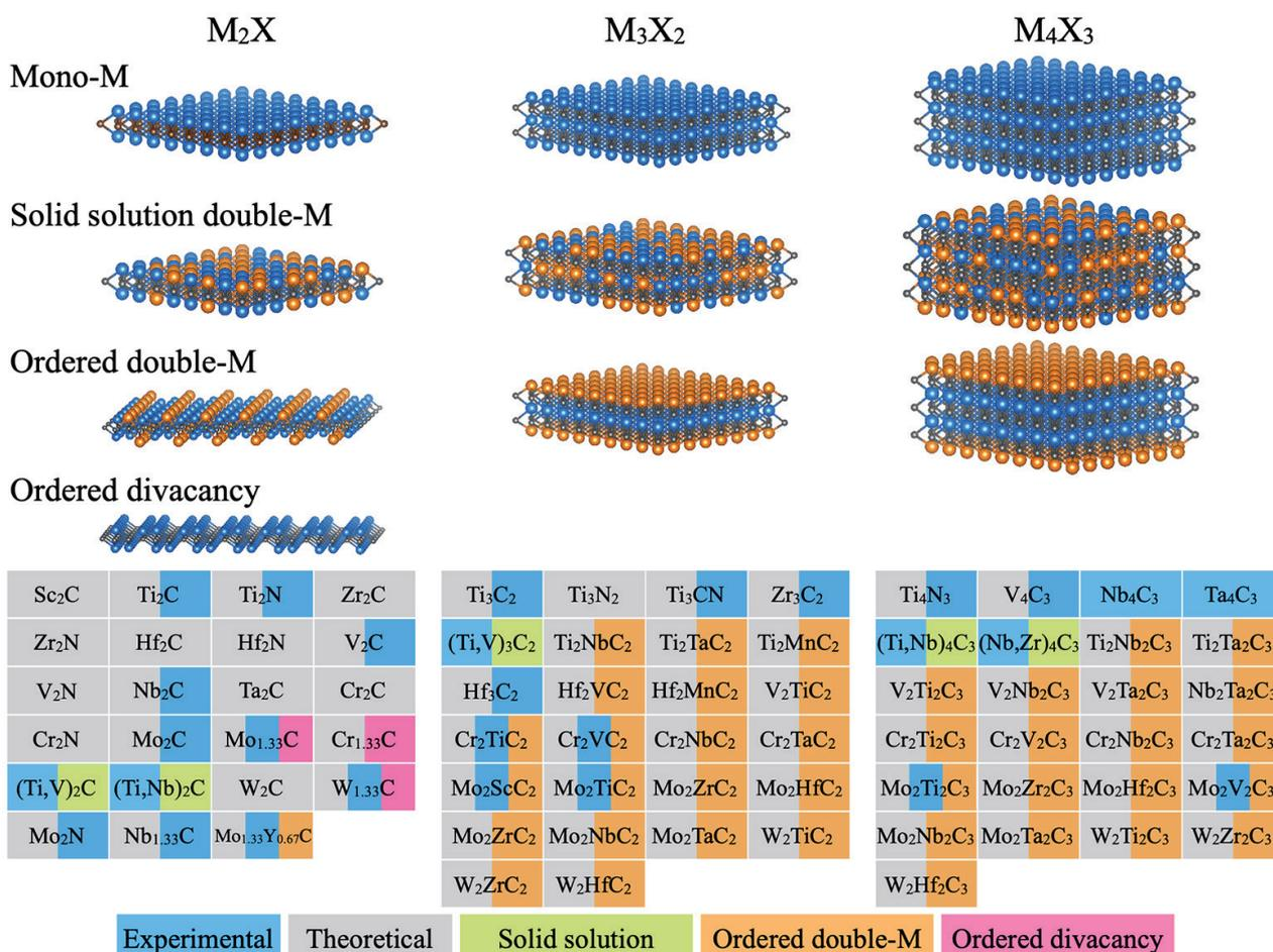
Figure 5. Chemical versatility of all existing MXene systems, including conventional  $M_{n+1}X_n$  ( $n = 1, 2, 3$ ), double-M solid solutions, out-of-plane ordered, in-plane ordered double-M, and divacancy ordered  $M_{n+1}X_n$  MXene systems. M and X elements are respectively represented by blue/orange and gray small spheres. Adapted from [51].
