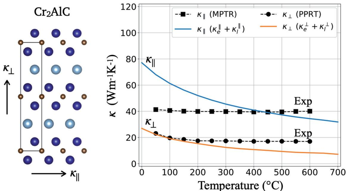
Figure 8. Total thermal conductivity obtained by summing the electronic and lattice contributions:  $k = k_e + k_l$ , compared to the experimental curves.
