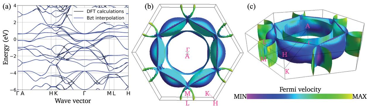
Figure 7. First-principles (a) electronic band structure of  $\text{Cr}_2\text{AlC}$ , with the Fermi level fixed as the reference of zero energy, and (b) and (c) Fermi surfaces computed using the Fermisurfer code [101] and color-coded depending on Fermi velocities.
