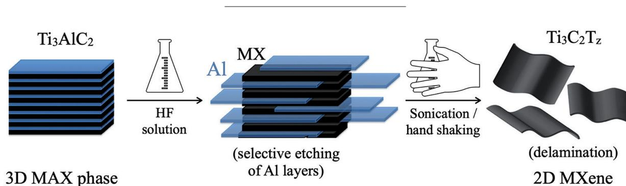
Figure 4. Schematic representation of the synthesis process of 2D MXenes, obtained from the selective etching of the Al planes from the parent 3D MAX phases when immersed in HF solution. Adapted from [50].
