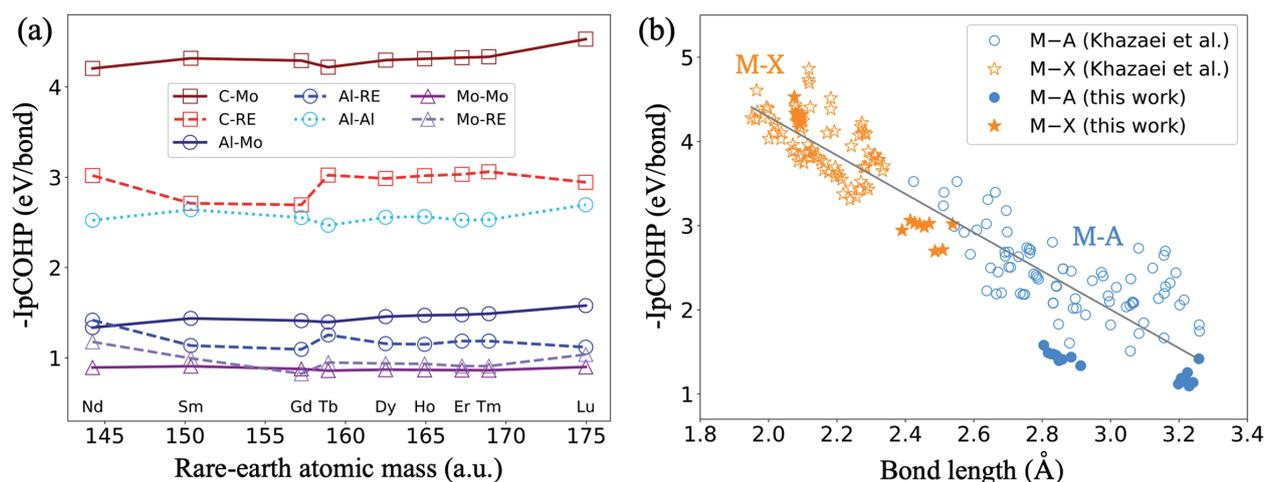
Figure 11. (a) Calculated integrated COHP values at the Fermi level as a function of the RE atomic mass. The relative order of bond strengths is almost unchanged with the RE atomic mass. (b) Integrated COHP for both M-A and M-X bonds for a series of 82 MAX phases (empty markers) [116] plus the 9 considered RE-i-MAX phases (full markers).
