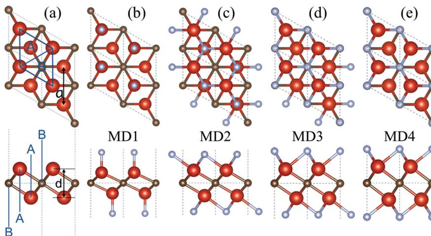
Figure 13. Atomic structures of (a) pristine  $V_2C$  and four models for terminated  $V_2CT_z$ : (b) MD1, (c) MD2, (d) MD3, and (e) MD4 - top and side views. V and C atoms are respectively in red and brown, while the functional groups ( $T = F, OH$ ) are in blue. In (a),  $a$  and  $d$  are the lattice constant and the layer thickness, respectively.
