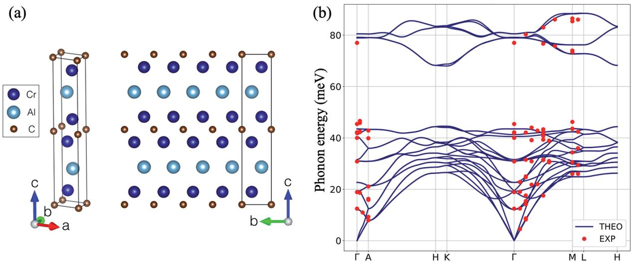
Figure 6. (a) Atomic structure of  $\text{Cr}_2\text{AlC}$  and (b) first-principles phonon spectrum and experimental phonon energy modes of  $\text{Cr}_2\text{AlC}$  along major crystallographic directions.
