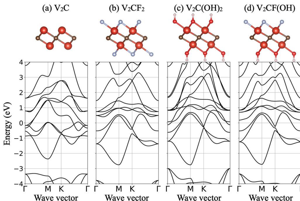
Figure 14. Electronic band structure of (a)  $V_2C$ , (b)  $V_2CF_2$ , (c)  $V_2C(OH)_2$ , and (d)  $V_2CF(OH)$  in their high-symmetric configuration. The Fermi level is fixed as the reference of zero energy.
