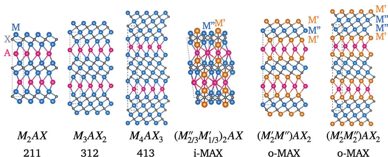
Figure 1. Atomic structure of existing MAX phases, including ternary  $M_{n+1}AX_n$  ( $n = 1, 2, 3$ ) phases, and quaternary in-plane ordered (i-MAX) and out-of-plane ordered (o-MAX) phases. The unit cells are represented with dashed lines and the M, A, and X elements are respectively represented by small blue/orange, pink, and gray spheres.
