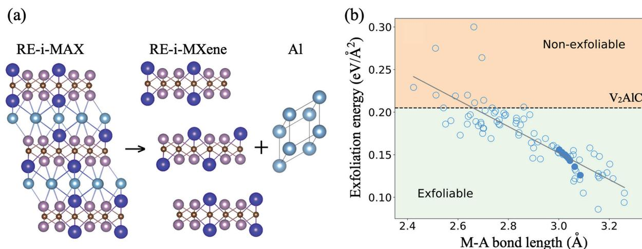
Figure 12. (a) Simplified representation of the exfoliation of a RE-i-MAX phase into RE-i-MXene, for which the exfoliation energy is obtained as a difference in energy of the products (RE-i-MXene + Al) and the reactant (RE-i-MAX). (b) Computed static exfoliation energy as a function of the bond length for a series of 82 MAX phases (empty markers) [116] plus the 9 considered RE-i-MAX phases (full markers).
