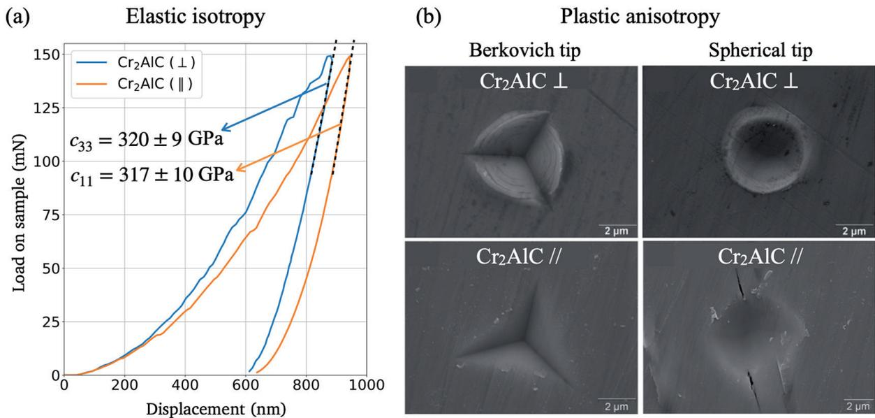
Figure 9. (a) Representative load-displacement curves from the nanoindentation of the top surface and sample side of a  $\text{Cr}_2\text{AlC}$  single crystal and (b) SEM images of the indentation marks of indent performed perpendicularly and parallel to the  $ab$ -plane, using a Berkovich or a spherical tip.
